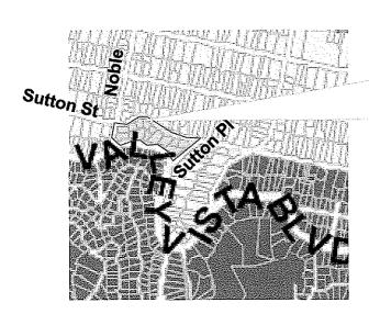
Area should remain classified as hillside because slope significantly exceeds 15% in several place around block, and several lots have existing retaining walls.
