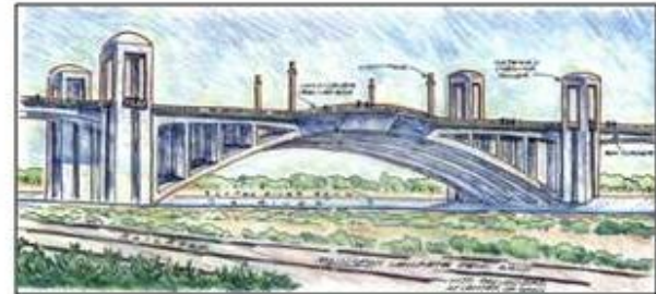
Alternative 5R – Concrete Deck Arch
