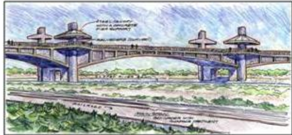
Alternative 2R – CIP Prestressed Concrete Box Girder
