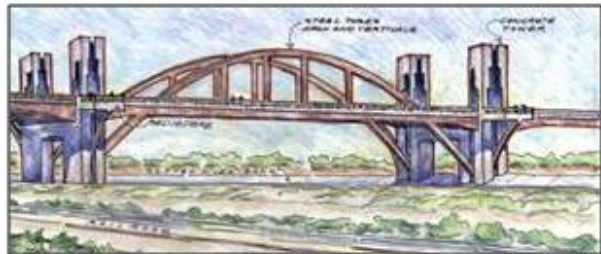
Alternative 9R – Steel Half Through Arch
