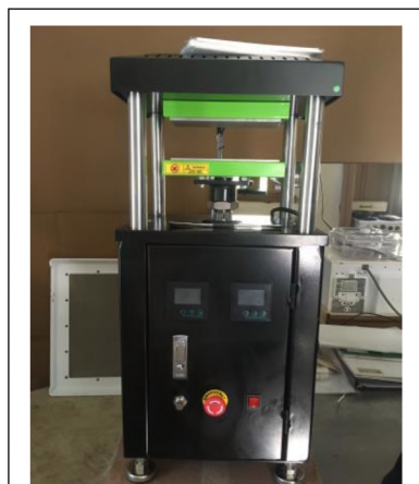
A rosin press consists of two heated plates which are pressed together at high pressure (typically between 300 to 600 psi) to convert hashish into rosin. This process is typically considered non-volatile manufacturing.
