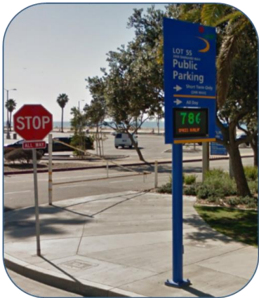
Figure 15. Vehicle Detection and Occupancy Digital Signage
