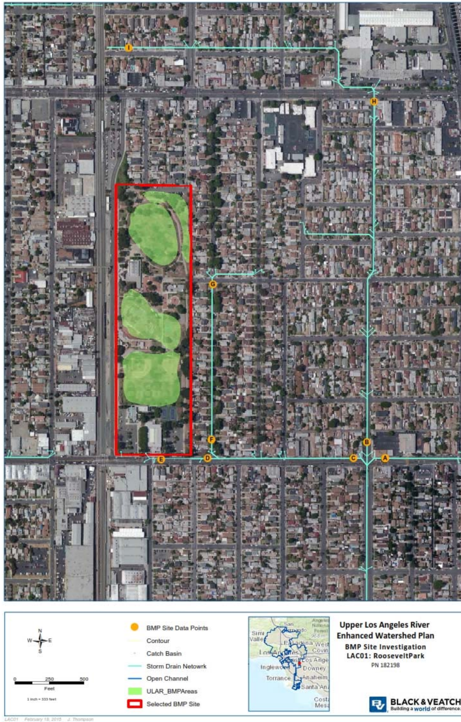
Figure 4-14. Roosevelt Park Subsurface Infiltration Drainage Area
