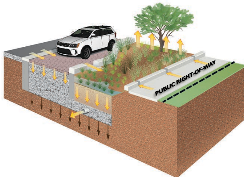
Figure 4.A-8. Typical distributed green street schematic (arrows indicate water pathways).
