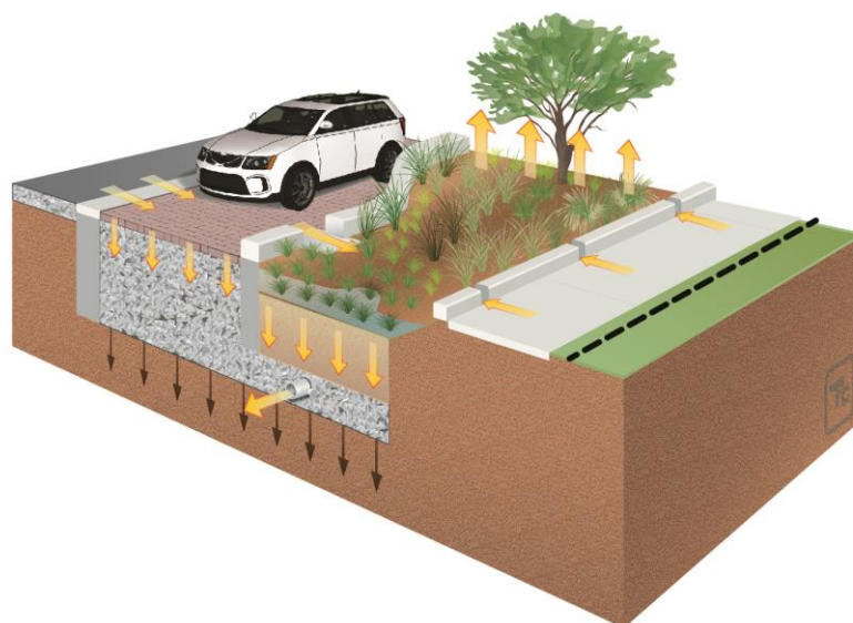
Figure 5-2 Conceptual schematic of green street/green infrastructure (arrows indicate water pathways)
