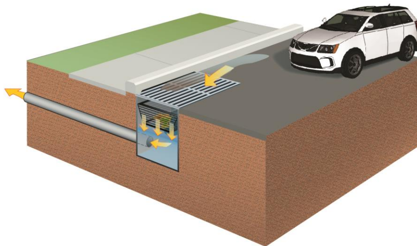
Figure 4.A-13. Typical distributed source control structural BMP (arrows indicate water pathways).
