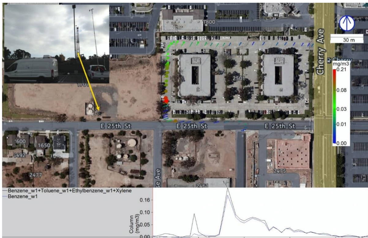
Figure 31. Emission from the drilling site at Walnut Avenue and Crescent Heights on October 16, 12:35-12:41 am. Both on October 15 and 16 high levels of benzene was measured downwind this site. This measurement showed BTEX levels up to 210 \mu\text{g}/\text{m}^3 , of which benzene 180 \mu\text{g}/\text{m}^3 . Wind speed was about 1-1.5 m/s, coming from WSW. Enclosed is a photo of the drilling rig, with the rig position indicated by the orange arrow, and with the FluxSense mobile lab in the foreground. Each measured spectrum is represented with a point, with color and size indicating the evaluated integrated vertical BTEX column according to the logarithmic color bar. The BTEX (black) and benzene (blue) column by distance driven through the plume is also shown in the lower part of the figure. A line from each point indicates the direction from which the wind is blowing.
