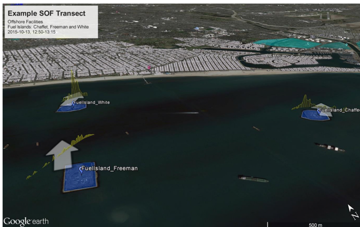
Figure 21. Example of SOF measurements of Fuel Islands outside Long Beach, 13 October 2015, 12:50-13:15. Alkane column is shown as a yellow curve with apparent height proportional to gas column (10 m equivalent to 1 mg/m 2 , max 35 mg/m 2 ). Wind direction during the measurement is indicated by the white arrow, measured with the FluxSense 10m wind mast. Map from Google Earth™ 2016.
