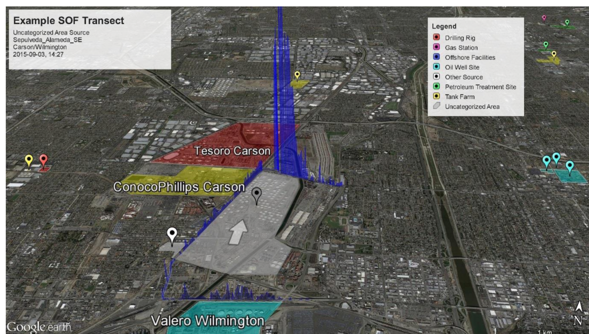
Figure 24. Example of a SOF measurement transect of the Uncategorized Area Source (gray shaded area) in Long Beach, 3 September 2015, 14:30. Also noted are large Refineries from Project-1 (names) and other surrounding sources from Project-2. Alkane column is shown as a blue curve with apparent height proportional to gas column (10 m equivalent to 1 mg/m 2 , max 400 mg/m 2 ). This particular transect gave 750 kg/h. Wind direction during the measurement is indicated by the white arrow. Map from Google Earth™ 2016.
