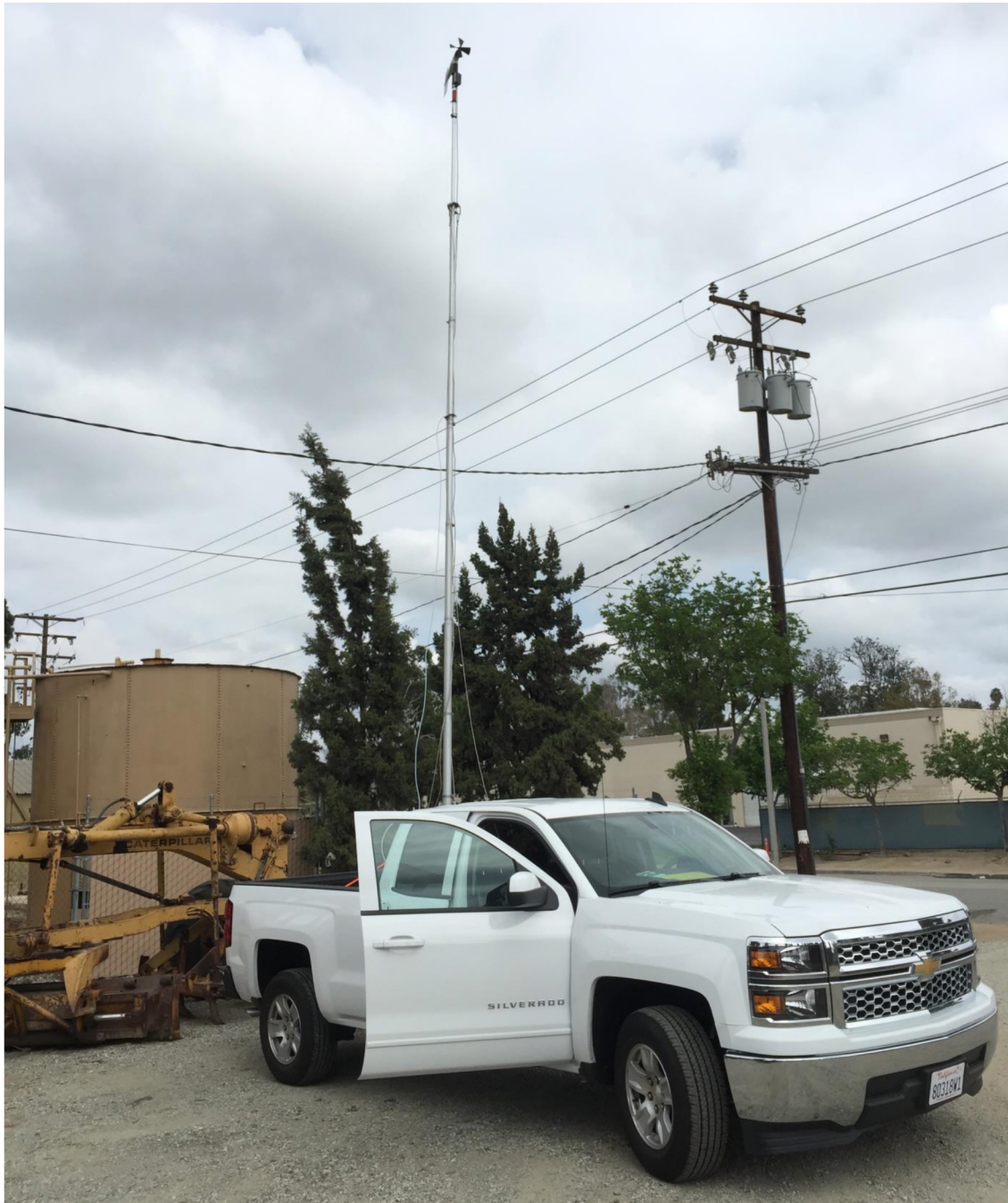
Figure 11. FluxSense mobile wind mast mounted on the bed of pick-up truck. An RM Young anemometer is used throughout the project. The mast could be erected from 3 to 10 m.
