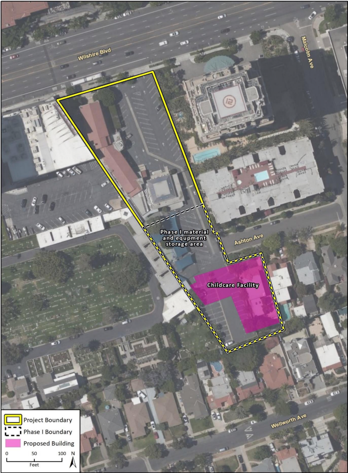
Figure 2-11 Phase I Staging
