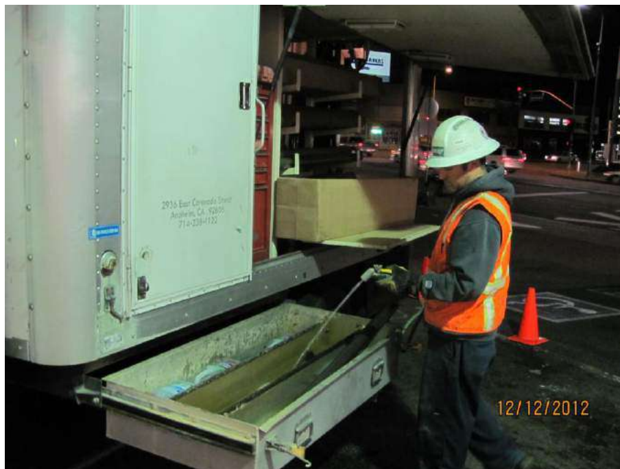
Decontamination of direct push rods
