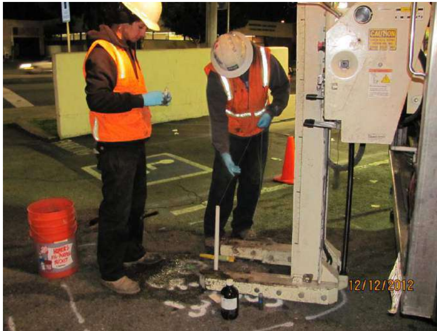
Grab groundwater sampling - Hydropunch™
