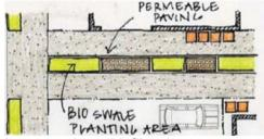
Incorporating a biofiltration system or bioswale can remove and oxiize organic gases
