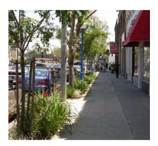
IMAGE B: Parkways can be designed to filter stormwater runoff from the street. If there is a raised curb around the parkway as in this example, the convenience strip next to the curb must be wider than 18 inches.
