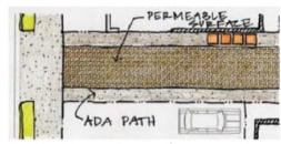
Permeable paving surfaces can be implemented to reduce stormwater runoff and increase infiltration rates
