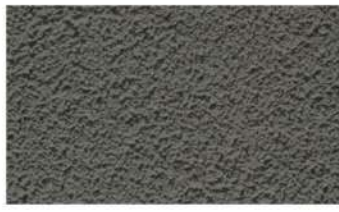
3 CEMENT PLASTER - DARK GREY - SAND FLOAT FINISH
