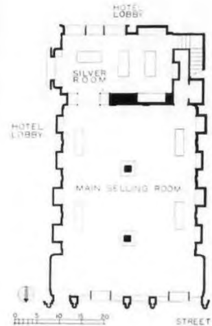
Above, plan of ground floor, showing connection with adjacent hotel lobby. Show windows, on both the lobby and the street sides, are subdivided into small display spaces, comparable in scale to objects displayed.
