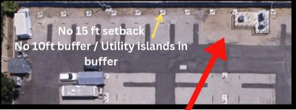
Utility islands and the 800-amp electrical distribution system have been constructed inside the required 15-foot setback and 10-foot landscaped buffer, a clear violation of Performance Standard #5
