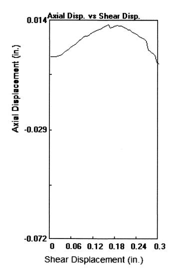
Parameters -Client: SCHICK Maximum Load Location: 1904 PRAUSS RD 1896 psf Job # 2499 Soil Type:AT Shear Displacement Sample: 1 Technician: BF at maximum Load **Boring: TP1** Axial Load: 1000 psf 0.1756 in. Depth: 10 ft. Shear Rate: 0.010 in./sec. File: 2499TP1121.dat Distance: 0.30 in. Date -6/26/2017 Stress at Max Def Stress at Max Disp 0.176 1896 0.296 552 Soil Labworks
