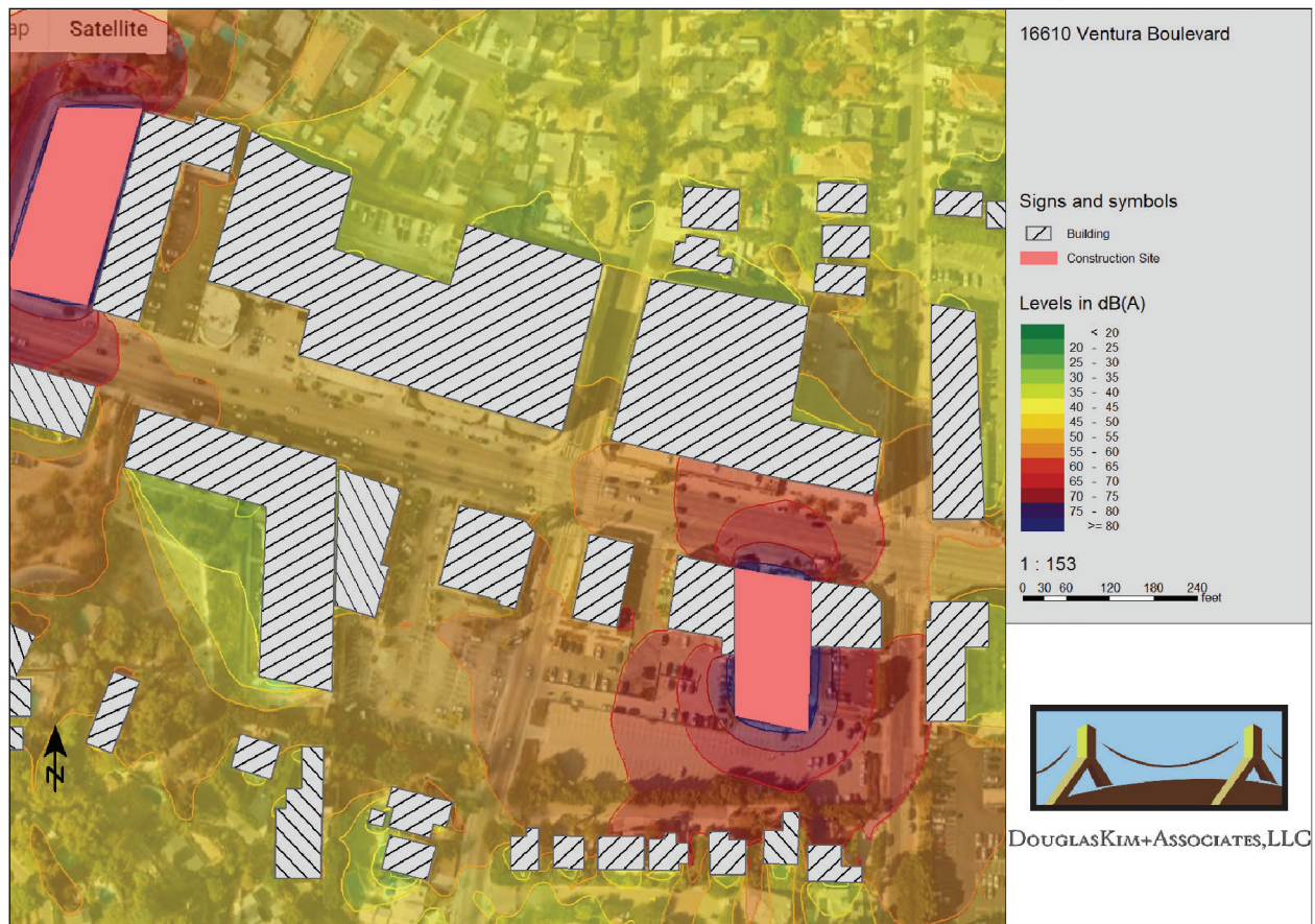
Figure 2-4 Construction Noise Sound Contours from Cumulative Development
