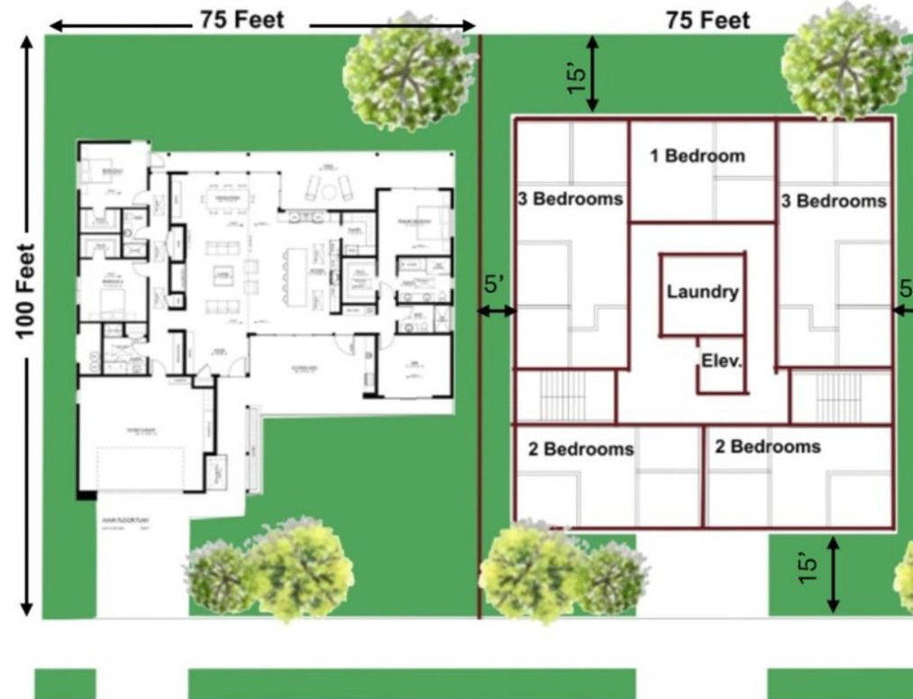
Typical Single-family house Option C1 Apartment Building 16 Units (floor 1 has 2-1 bed units in lieu of a 3 bedroom unit) 4 Stories ( 3 above parking)
