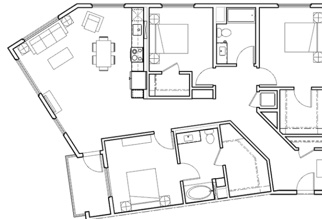
Plan D2 3 Bedroom / 2 Bath 1,565 sf Habitable Rooms for Parking: >3 Habitable Rooms for Open Space : >3
