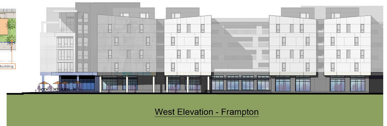
West Elevation - Frampton Exterior Wall Area = 2,640 sf. Approx. Storefront Area Provided = 1,450 sf. (55%) Approx.
