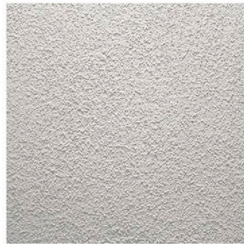
1. EXT. CEMENT PLASTER 20/30 SAND FINISH
