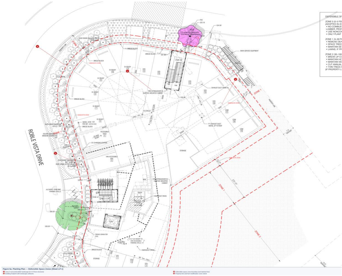
Figure 5a – Planting Plan — Defensible Space Zones (Sheet LP-1). Callouts identify: (1) Zone 0 noncombustible hardscape (0–5 ft from structure), (2) defensible space zone boundary (red dashed line), (3) building footprint with landscape setbacks, (4) property line and fuel modification zone extent.
