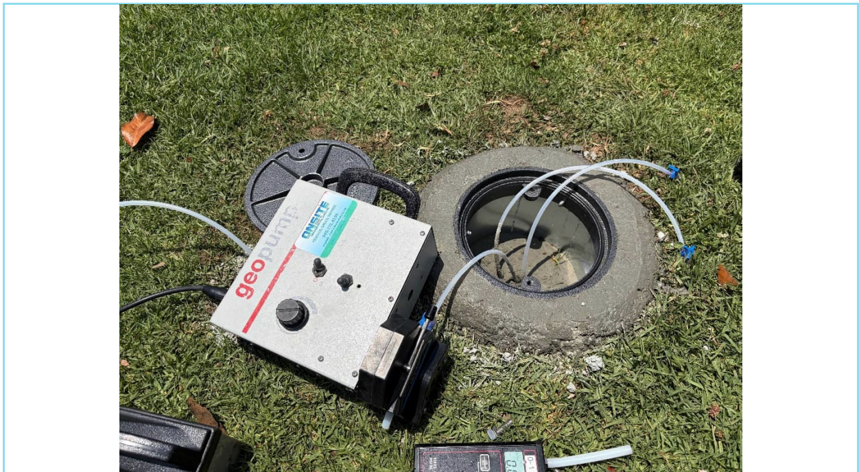
Photo 4: Purging and sampling at SGP-2.
